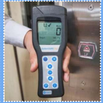
Applying a self-disinfecting coating (SDST) to lift buttons kills germs and prevents them from breeding. After application, the ATP reading of bacteria count drops to zero
